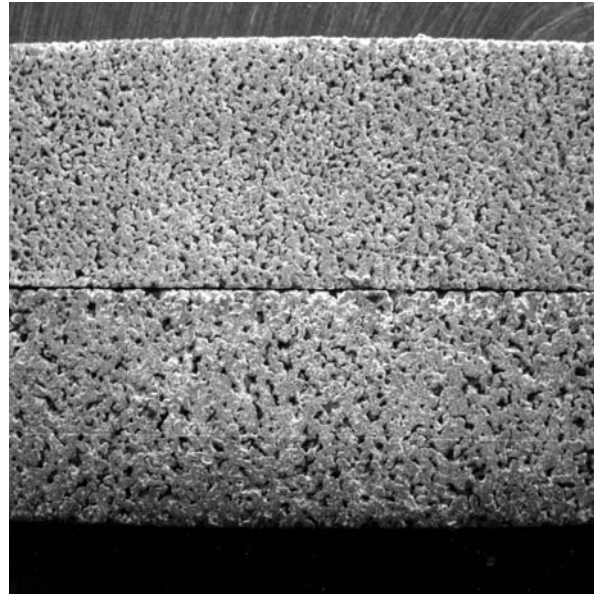
Figure 7. SEM image of EDM'ed surfaces of porous materials manufactured using different processes. (Top)– uniform porosity was maintained. (Bottom)–uneven pore distribution.
